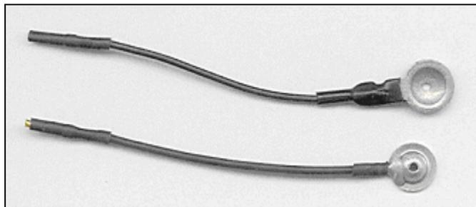
Figure 10 – Typical Silver/Silver Chloride (Ag/AgCl) Electrodes
