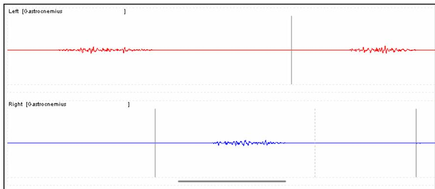
Figure 8 - EMG recorded at too low a level is difficult to observe or analyze.
