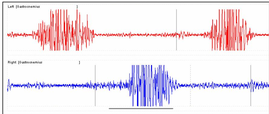
Figure 9 - EMG recorded at too high a level is distorted and provides limited information.
