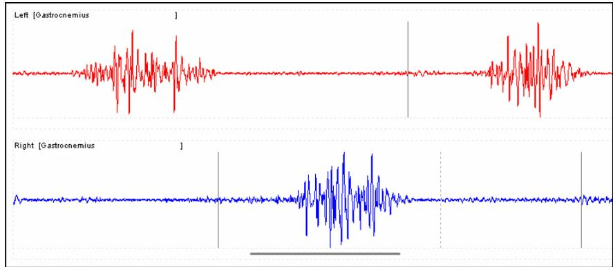
Figure 7 - EMG recorded at the correct level is large enough to be analyzed but does not clip.
