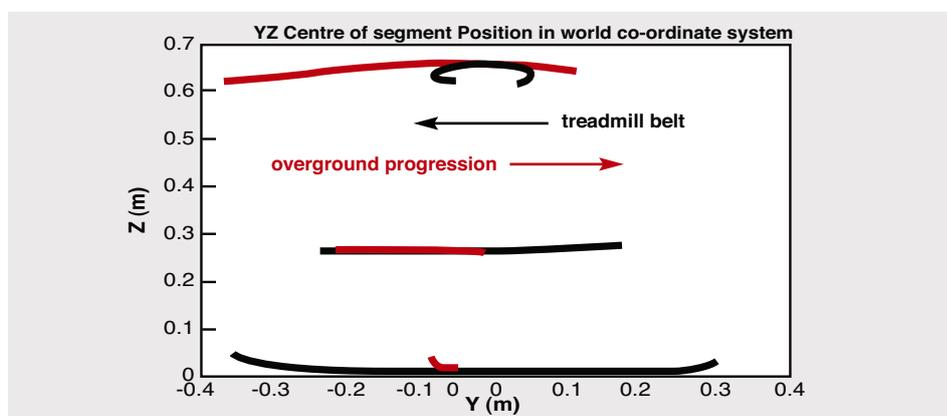
**Figure 3.** Movement of the foot, shank, thigh segments during both treadmill and over-ground gait.
