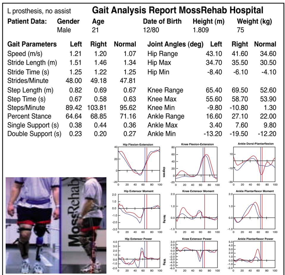
Following are examples of component selection differences and height adjustments with resulting gait improvements as documented by 3D gait analysis. Data collected at Moss Rehab from a transfemoral amputee using a 7 bar multi-ax is knee (Century) and a micro processor controlled C-leg (Otto-Bock).
