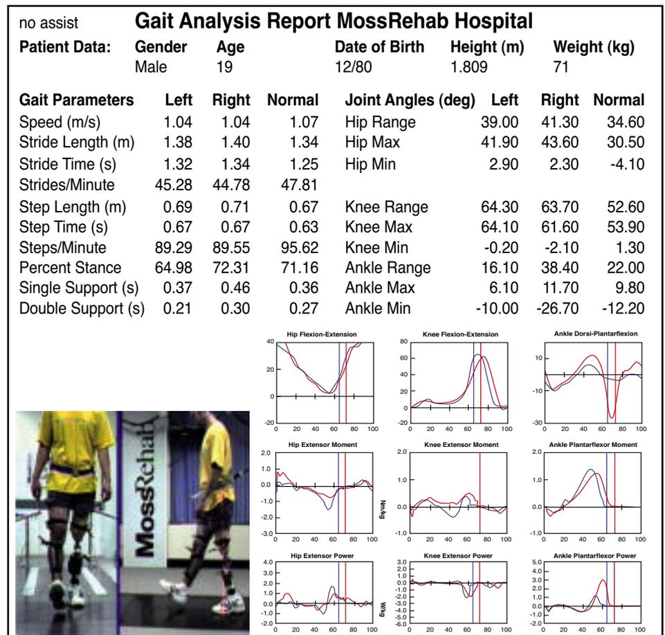
stance and swing times for each foot as well as stride lengths and step lengths. By comparing the two sides, measures of symmetry can be obtained to determine the extent of unilateral impairment and the impact of interventions on symmetry of walking.
