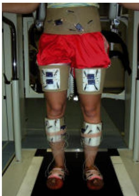
**Figure 1.** Codamotion markers are placed on subject's legs and pelvis to track motion during treadmill and over-ground walking trials.
